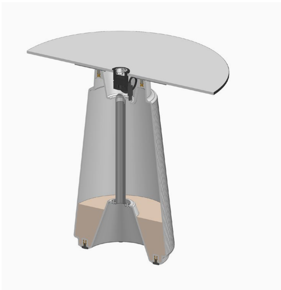
Electrified column with an inner tube made of steel with a diameter of 140 mm and bolted to the bottom of the column.
