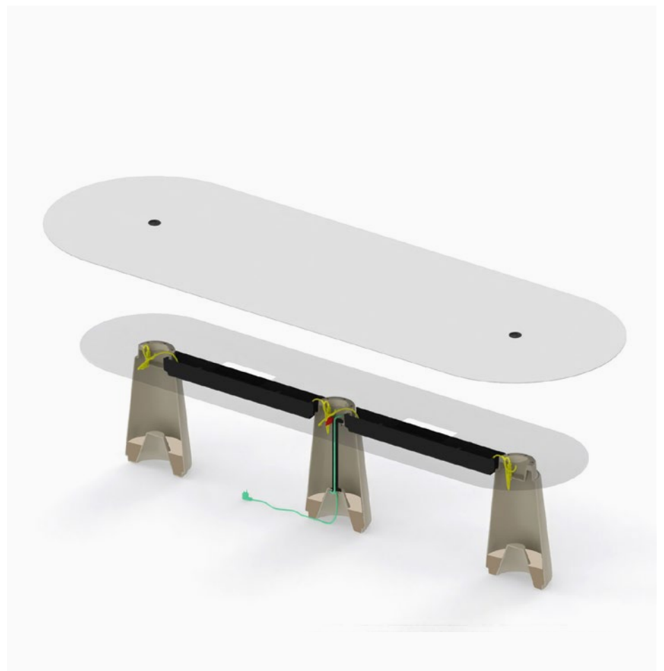
Integrated electrical management consisting of an electrified column and a two cables tray connecting the three columns. One of the three columns is electrified with an inner tube made of steel with a diameter of 40 mm and bolted to the bottom of the column. The electrification tray is made of folded sheet steel with a thickness of 3 mm.
